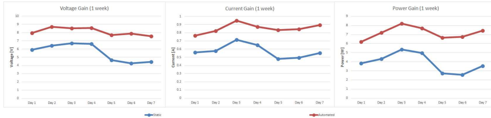
Fig. 4.9. Voltage, Current, and Power Gain of Automated Panel (red color) over Static Variant (blue color).
