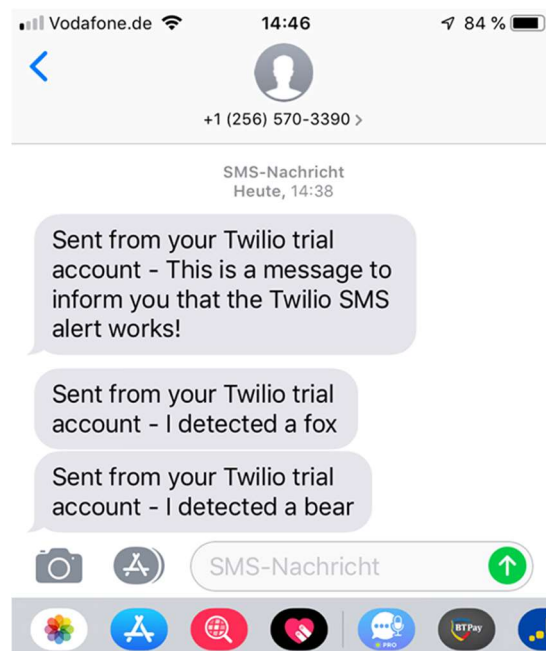
Fig. 4.29. Example of an automated SMS alert using Twilio API.
