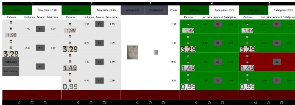
Fig. 3.5. Summarized Android GUI view of the proposed Receipt Fraud application: Products (Items) View (1 and 2); Receipt View (3); Products (Items) View after price comparison between Receipt and Products was made and Price is equivalent (4) or not equivalent (5).
